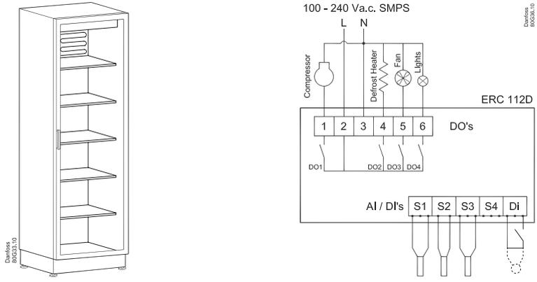
Note: this is a typical (default) wiring diagram since both inputs (AI/DI's) and outputs (DO's) can be assigned differently. Please see "AI/", assignment
